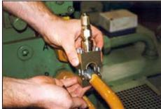
•Clamp the valve mount to the pipe
