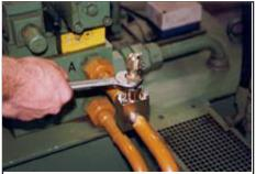
•Using an open jawed wrench (without extension), screw back head joint in counter-clockwise direction.
